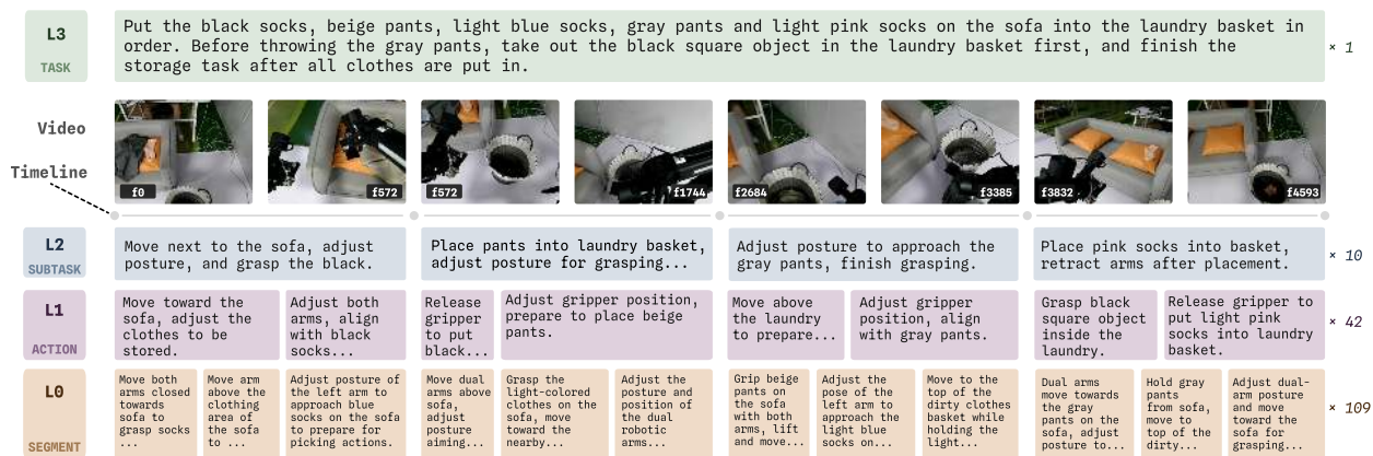
Figure 12 Four-level caption tracks for a single episode. The visualization stacks the four core lanes shown in the figure: Task (L3), Subtask (L2), Action (L1), and Segment (L0), aligned to the video timeline.
