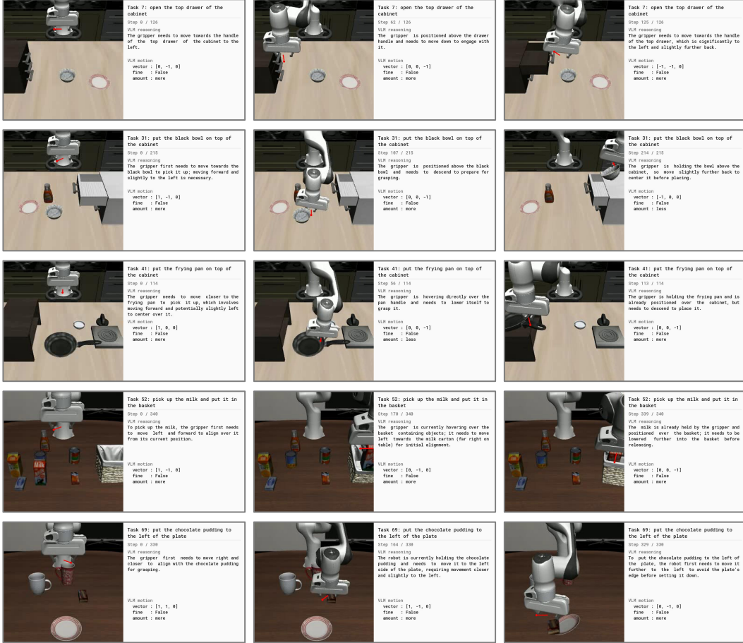
Fig. 19: Example outputs of VLM steering in LIBERO. Red indicates the direction suggested by the VLM.
