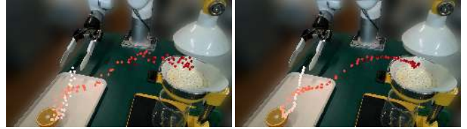
Fig. 10. Representative trajectories of Po-Dec (left) and ZPRL (right) from the same initial state. Dots denote recorded EE positions projected onto the image frame. Darker dots indicate later timesteps along the trajectory.
