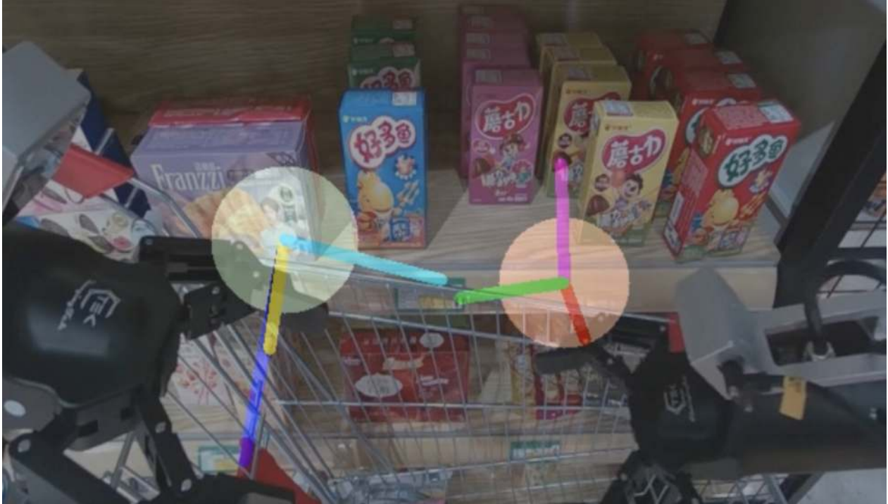
Figure 6 Vision-action alignment verification. Calibrated action signals are rendered as semi-transparent action maps and overlaid onto video frames. Samples with spatial deviation between projected trajectories and observed robot motion are identified and removed.
