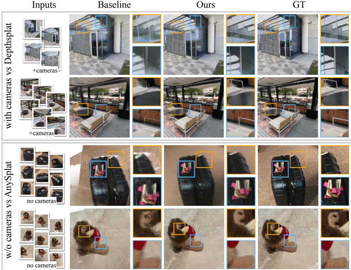
Figure A2. Qualitative comparison vs Feed-forward 3DGS. Our model more accurately represents reflective areas (mirror, top row and table, second row) and thin structures (metal rod, top row and chair arm, second row). The global, latent representation leads to better surface alignment (suitcase handle, third row and teddy bear, bottom row) and is more robust to occlusions (floor, third row).
