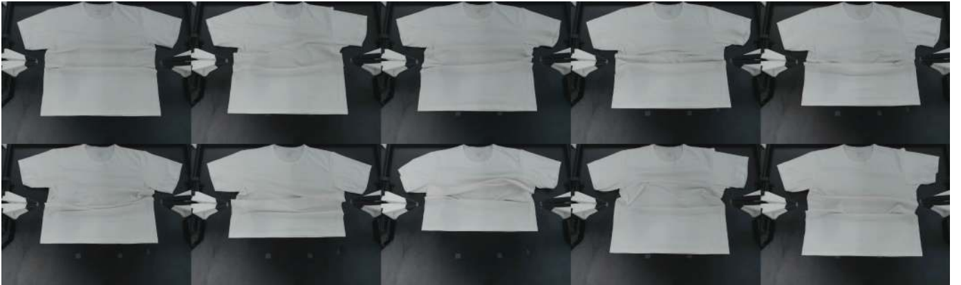
Fig. 10: Initial states for “fold shirt” task evaluations. The bottom edge of the shirt varies by 15 cm along the tabletop’s vertical axis across different trials.
