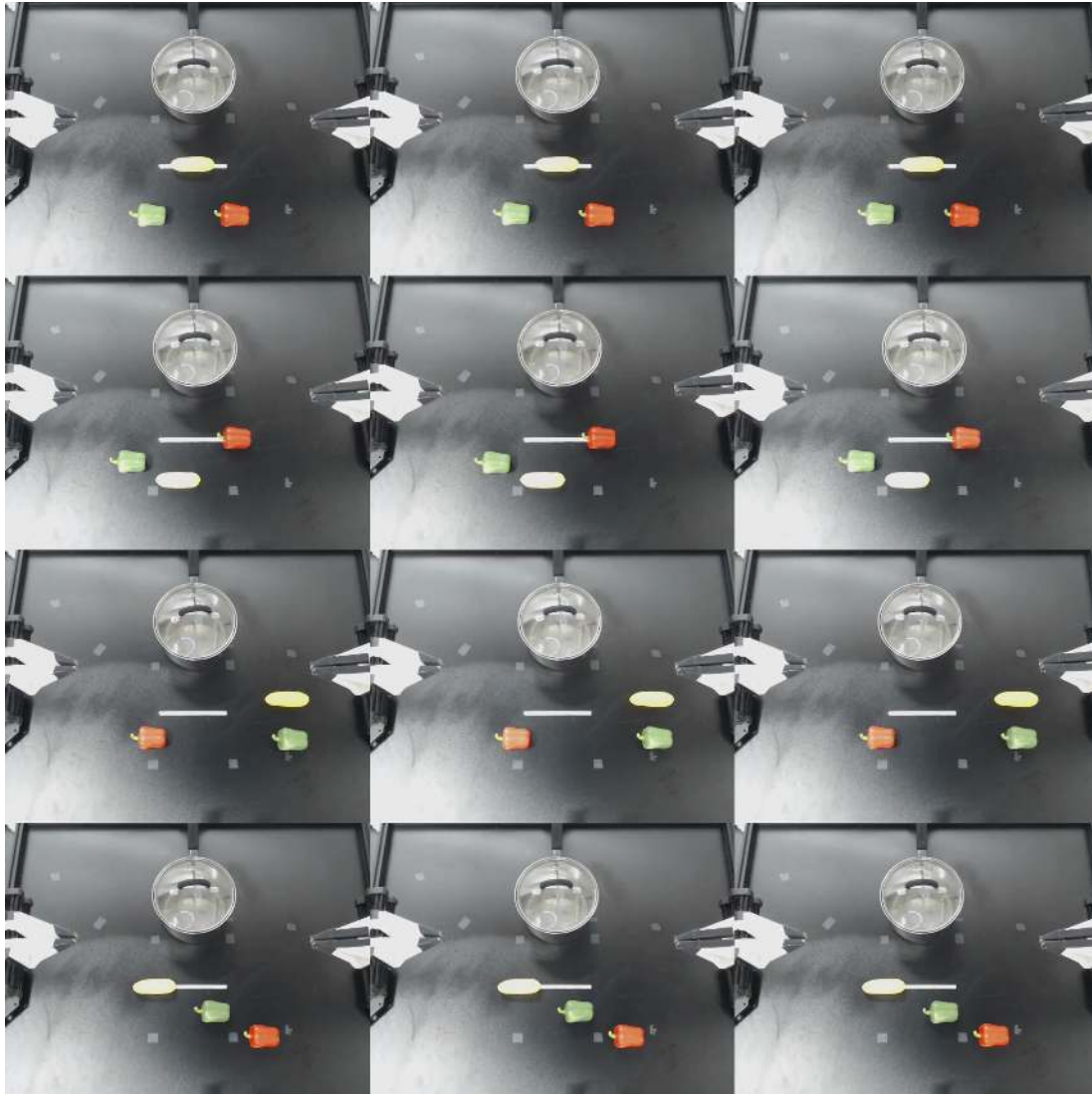
Fig. 12: Initial states for “put X into pot” task evaluations (in-distribution version). Food object positions vary by 15 cm vertically and 40 cm horizontally across trials, while the pot remains stationary. Each grid row presents three identical initial states, as we cycle through the three target objects (“green pepper”, “red pepper”, and “yellow corn”) using the same initial configurations before we move on to the next set of initial configurations. (Refer to Figure 13 for the out-of-distribution version of this task.)
